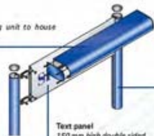
Module Plus post ø 60mm with fabricated panel inserts.
